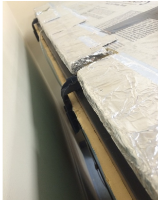
Foam top with cutouts for hose clamps
